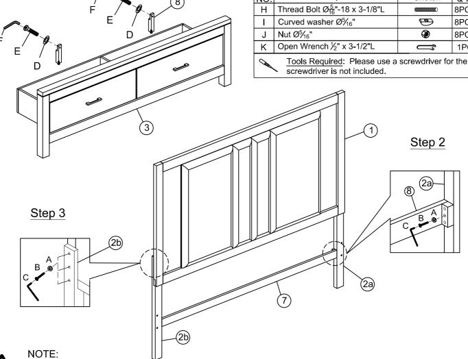
Must tighten screws periodically with use. Screws will become loose, check tightness of all screws every 6-8 weeks.
