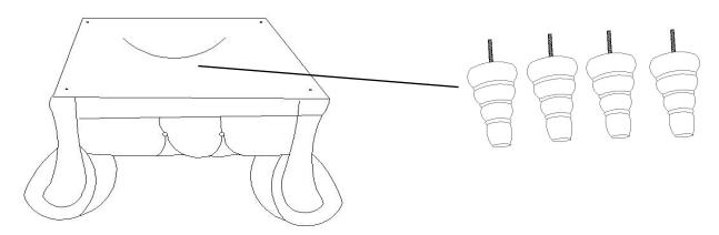
**Step#2** Align the legs to the pre-drilled holes as shown in drawing, rotate the legs in order to tighten it in secure and proper position.
