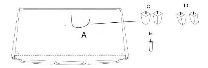
Step#2 Align the legs to the pre-drilled holes as shown in drawing, rotate to tighten it.
