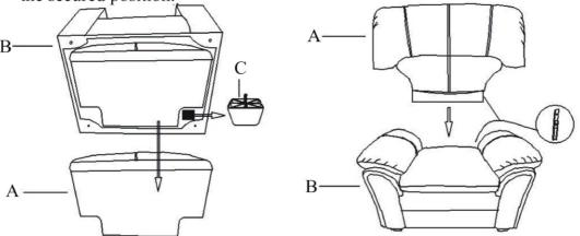
Step2. Align the bun foot to the bottom, insert and rotate the bolts then tighten it.
