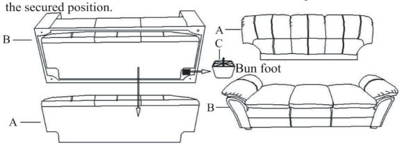
Step2. Align the bun foot to the bottom, insert and rotate the bolts then tighten it.
