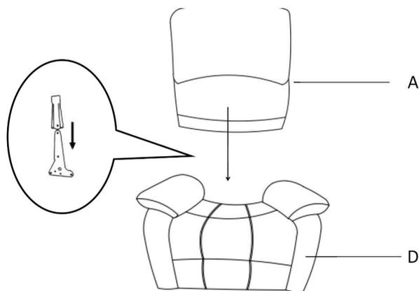
**Step 3.** Insert the LSF ear and RSF ear to the back rest and make sure it is secured in position.
