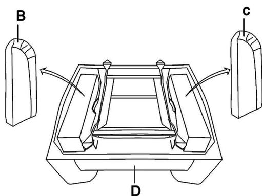
**Step 2.** Align the female brackets at the back rest onto the male brackets at the seat, insert and push to the end, make sure the brackets are secured in position.
