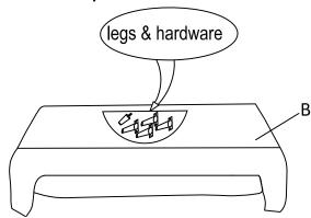
Step #2 Align the legs to the pre-drilled holes, insert the bolts then tighten with Allen key.
