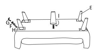
Step #3 Two person assembly is recommended for the back rest. Align both side of male brackets at back rest to be levelled onto the top of the female brackets at inner of seat frame. Insert the back rest and push down slowly to make sure the brackets are connected to each other. Slowly push to the end and make sure back rest is secured in position.
