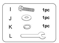
Attach the seat cushion frame (B) to the chair back (A) with 4pcs bolt (G), 4pcs flat washer(J), 4 pcs spring washer (K) then tighten using wrench (L).
