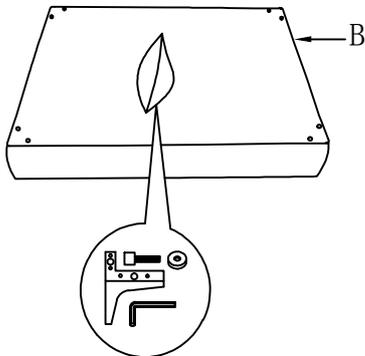
Step 2. Align the legs onto the pre-drilled holes at the bottom of the unit, insert bolts and washers then tighten with Allen Key.
