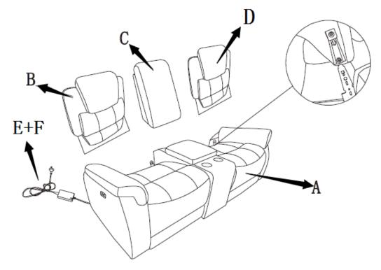
**STEP#2** Attach the adapter and power cord to the position as shown in the drawing properly.
