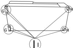
Step #3 Align and connect metal hooks to assemble the sectional.
