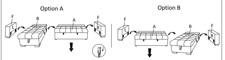
Step #4 Align and insert all brackets on back rest to seat, push to the end to secure in place properly.
