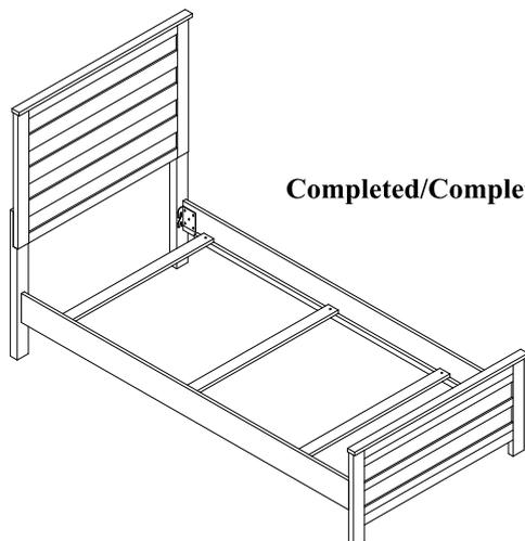
**\*\*DO NOT TIGHTEN BOLTS UNTIL COMPLETELY ASSEMBLED**
