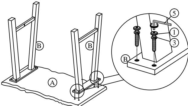
*DO NOT TIGHTEN BOLTS UNTIL COMPLETELY ASSEMBLED.
