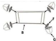
Step 2. Insert back rail into back rest and make sure it's secured in position.
