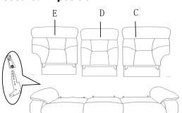
Step 2. Insert the ear to the back rest and make sure it is secured in position.
