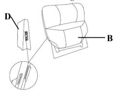
STEP# 2 Align the female brackets at the back onto the male brackets at the seat, insert back rest to the seat and make sure it is fixed in position securely.
