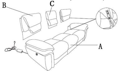
Note: Press down seat back gently until you hear a "click" to make sure it is locked in place. STEP#2
