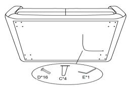
Step 2. Align the legs onto the pre-drilled holes at the bottom of unit, insert bolts then tighten with Allen key.
