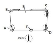
Step #3 Connect 2 seater and chaise with pre-assembled metal brackets.
