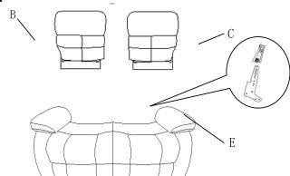
Step 2. Insert the LSF ear and RSF ear to the back rest and make sure it is secured in position. make sure the brackets are secured in position.
