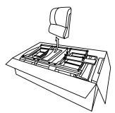
Step 3. Align the female brackets at the back onto the male brackets at the seat, insert and push to the end, make sure the brackets are secured in position.
