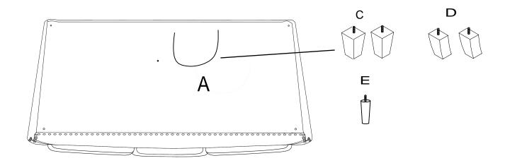
Step#2 Align the legs to the pre-drilled holes as shown in drawing, rotate to tighten it.
