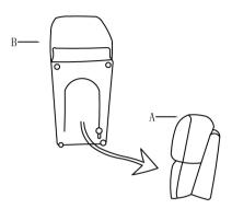
Step 2. Align the female brackets at the back rest onto the male brackets at the seat, insert and push to the end, make sure the brackets are secured in position.
