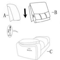
Step 1. Insert the LSF ear to the back rest and make sure it is secured in position.
