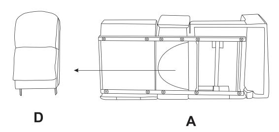
Step 2. Align the female brackets at the back rest onto the male brackets at the seat, insert and push to the end, make sure the brackets are secured in position.
