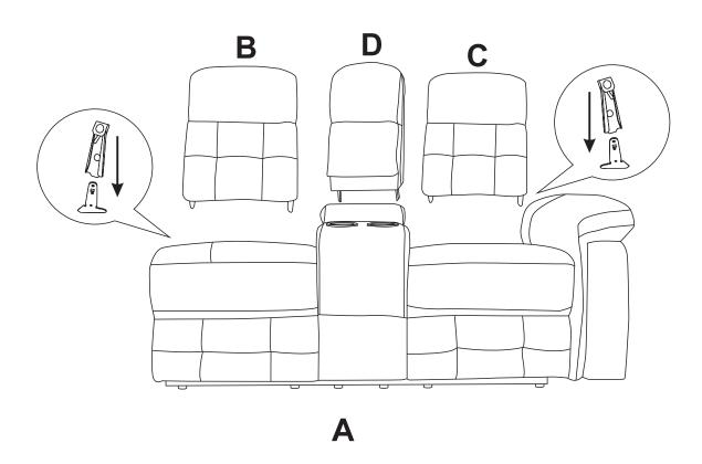
Step 3. Insert the RSF ear to the back rest and make sure it is secured in position.
