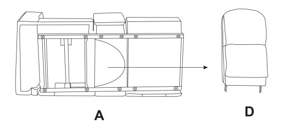
Step 2. Align the female brackets at the back rest onto the male brackets at the seat, insert and push to the end, make sure the brackets are secured in position.
