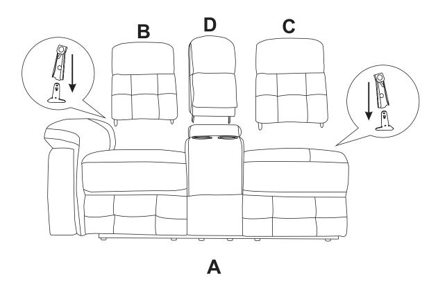
Step 3. Insert the LSF ear to the back rest and make sure it is secured in position.
