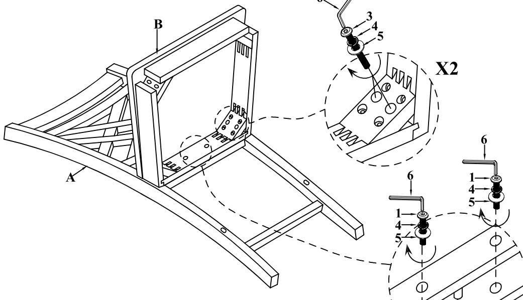
DO NOT TIGHTEN BOLTS UNTIL COMPLETELY ASSEMBLED.
