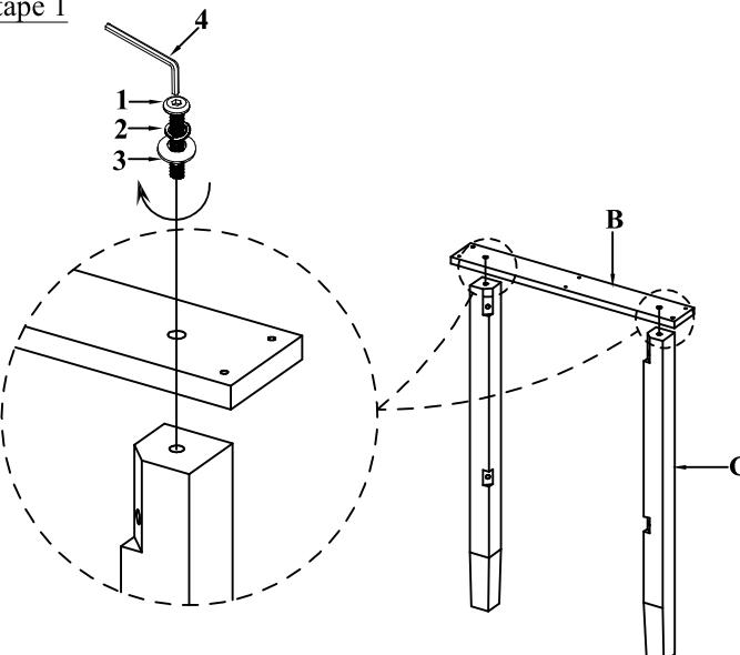
DO NOT TIGHTEN BOLTS UNTIL COMPLETELY ASSEMBLED.
