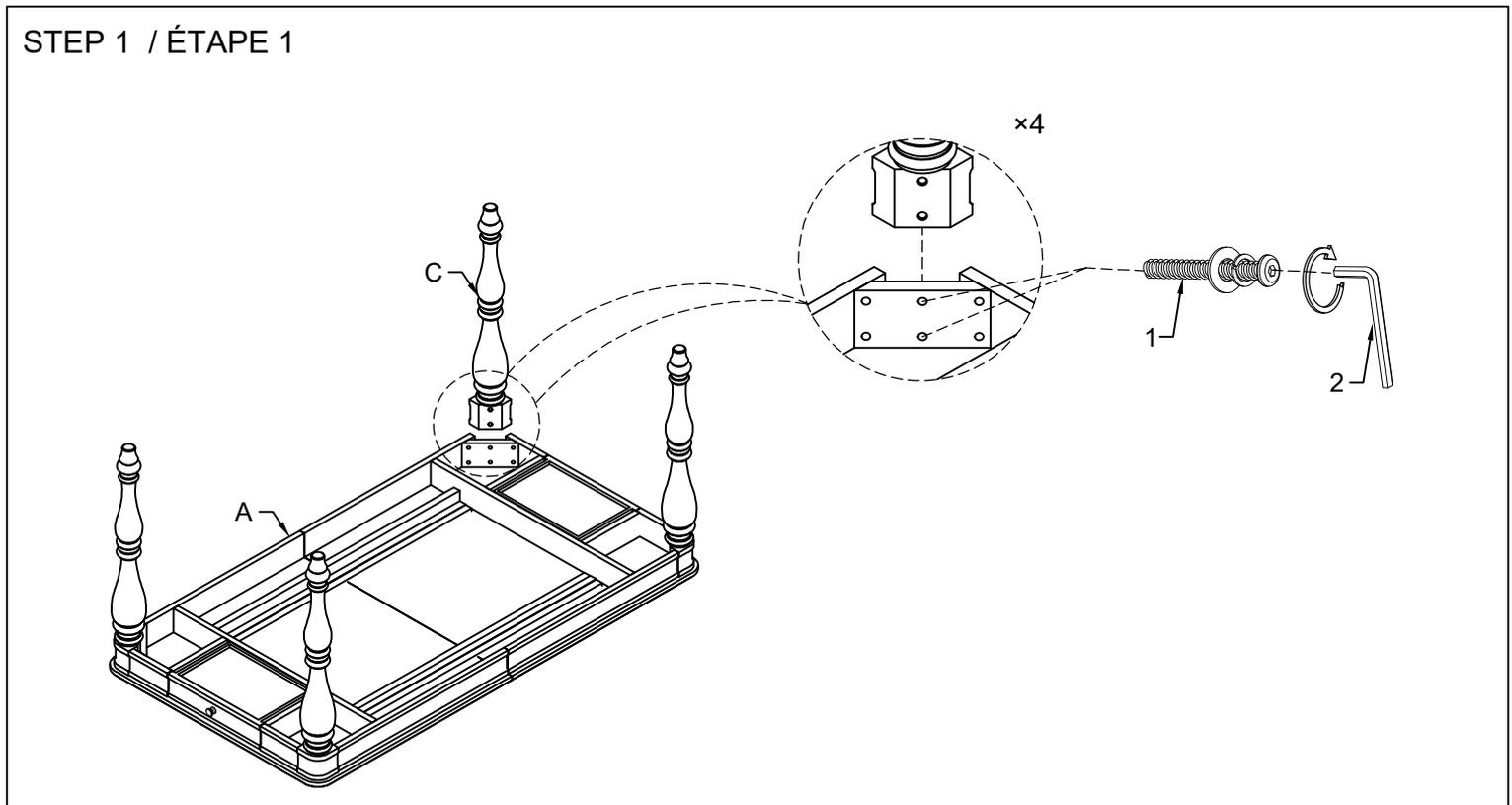
DO NOT TIGHTEN BOLTS UNTIL COMPLETELY ASSEMBLED.
