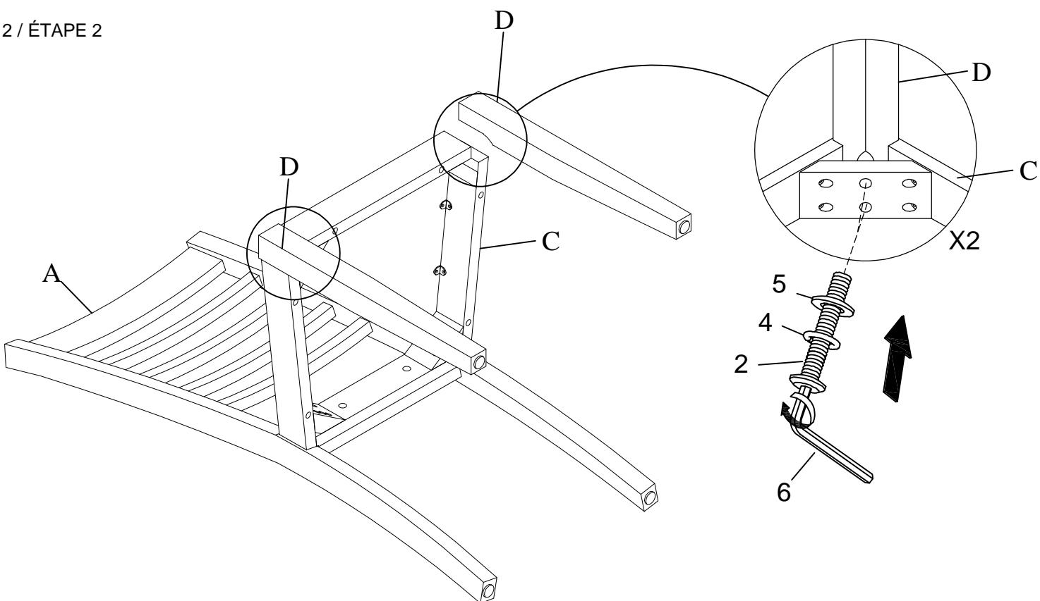
DO NOT TIGHTEN BOLTS UNTIL COMPLETELY ASSEMBLED.
