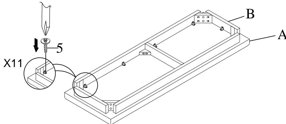
DO NOT TIGHTEN BOLTS UNTIL COMPLETELY ASSEMBLED.
