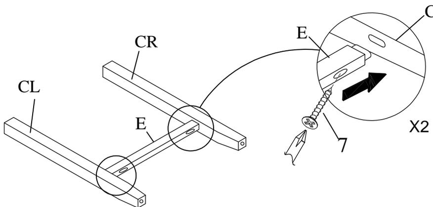
DO NOT TIGHTEN SCREWS AND BOLTS UNTIL COMPLETELY ASSEMBLED.
