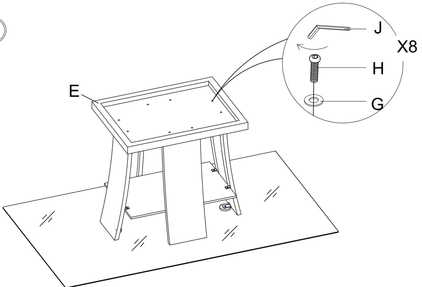
DO NOT TIGHTEN BOLTS UNTIL COMPLETELY ASSEMBLED.
