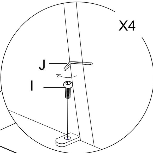
DO NOT TIGHTEN BOLTS UNTIL COMPLETELY ASSEMBLED.
