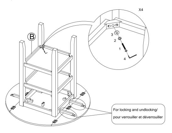
DO NOT TIGHTEN BOLTS UNTIL COMPLETELY ASSEMBLED.
