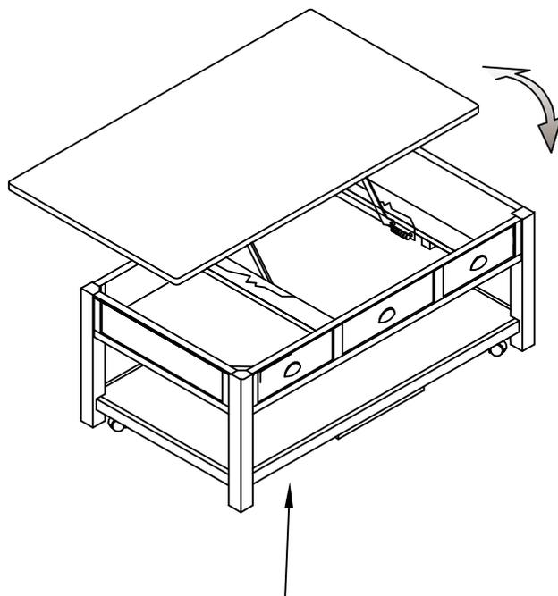
Please make sure the lower panel is assembled on the correct side with weight support to prevent tilting.
