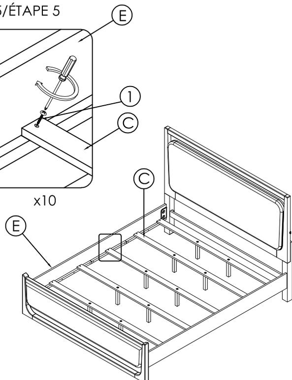
DO NOT TIGHTEN BOLTS UNTIL COMPLETELY ASSEMBLED/
