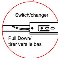
Pull the Drawer(9) to fully extend rail to see the switch. Then, using both hands pull UP the switch on left hand side and pull DOWN the switch on right hand side. Then remove the drawer from the Drawer Bottom Panel (10).
