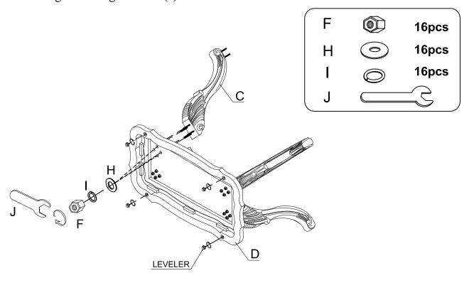
Attach the mounting plate (E) to the pedestal (C) with 8 pcs hex nut (F), 8 pcs flat washer(H), then tighten using wrench (J).
