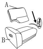
Step 2. Insert the LSF ear to the back rest and make sure it is secured in position
