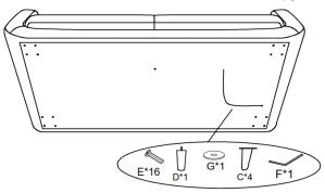
Step 2. Align the legs onto the pre-drilled holes at the bottom of unit, insert bolts then tighten with Allen key.
