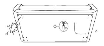
Step 3. Align the female brackets at the back rest onto the male brackets at the seat,insert and push to the end, make sure the brackets are secured in position.
