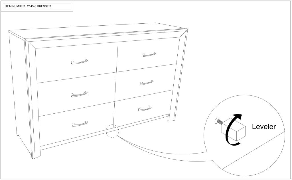
NOTE: AFTER A FEW DAYS OF ASSEMBLY, IT WILL HAVE ACCLIMATIZED TO THE ENVIRONMENT. PLEASE TIGHTEN ALL HARDWARE. CHECK TIGHTNESS OF ALL SCREWS EVERY 6-8 WEEKS.
