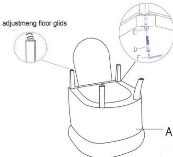
**Step 3** Check all the bolts are tighten securely in position, put the dust cover back to the position. Upright the chair and make sure the chair is stable.
