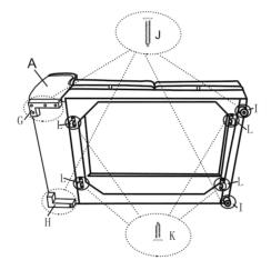
Step #3 Align and connect metal hooks to assemble the sectional.
