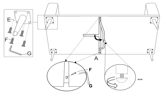
\*\*\* Adjust the sofa height to your preference by loosening or tightening the adjustable nut.
